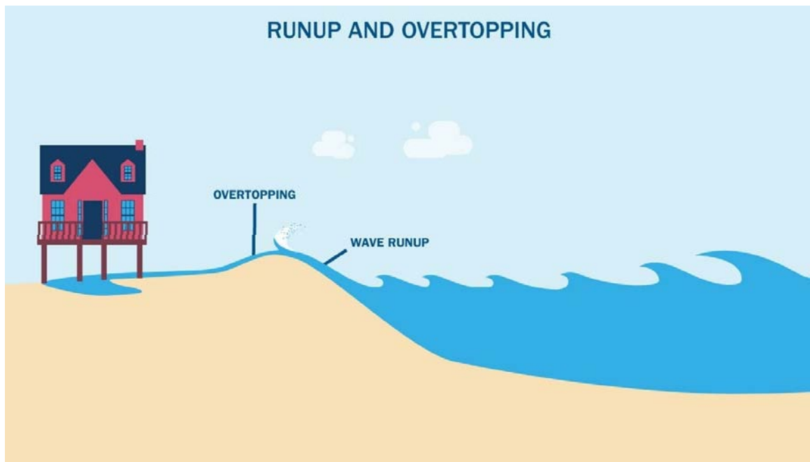
Figure 5b: Wave Overtopping Schematic
